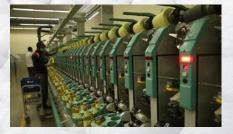
Auto-cone winding machinery from well-known company Savio from Italy serves to produce high quality yarn packages with latest Loepfe Zenit® yarn clearer.
