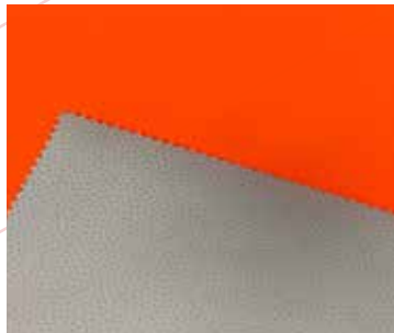
Hi vis orange recycled polyester with FR PU +PTFE lamination 200 GSM
